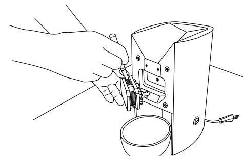
The crushing unit can now be removed. All parts can be cleaned with a brush.
